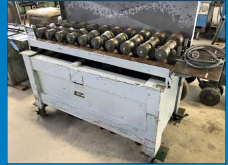
20 Ga. Lockformer 10-Stand Small and Large S and Drive Machine
