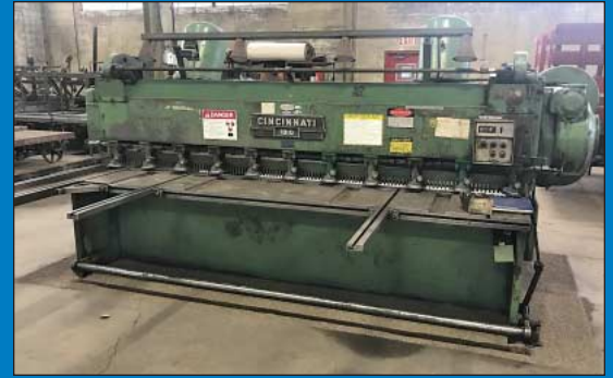
1/4" X 10' Cincinnati Model 1810 Mechanical Shear
