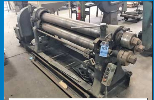
5/16" X 60" Hendley and Whitmore Model 4-D Plate Bending Rolls
