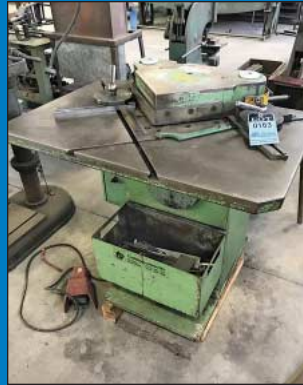
220 MM X 220 MM Boschert Model LB12PN4 Corner Notcher
