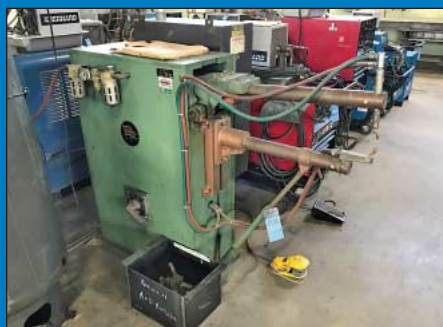
75 KVA Weltronic Model 2CR75A24 Spot Welder
