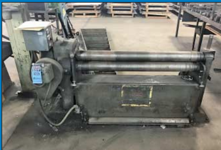
48" X 12 Ga. Reed Model 450 Plate Bending Machine
