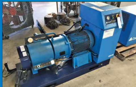
20 HP Compair Model HV-15 Air Compressor and Dryer
