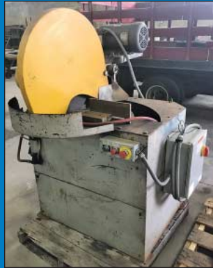
20" Everett Model 20MIT22 Mitre Abrasive Cut Off Saw
