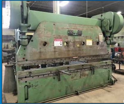
150/225 Ton X 12' Cincinnati Model 9 Series Mechanical Press Brake
