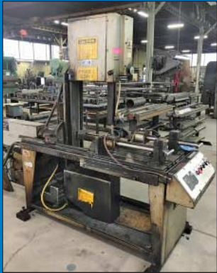
18" X 22" Hem Model V100LM Tilt Frame Vertical Band Saw
